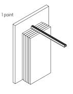
Movable/operable partition walls supported on tracks from above without any floor tracks.
